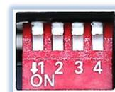
**After each Dip-switch-change a power-reset of the video interface has to be performed!**
