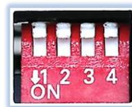
Dip position down is ON and position up is OFF.
