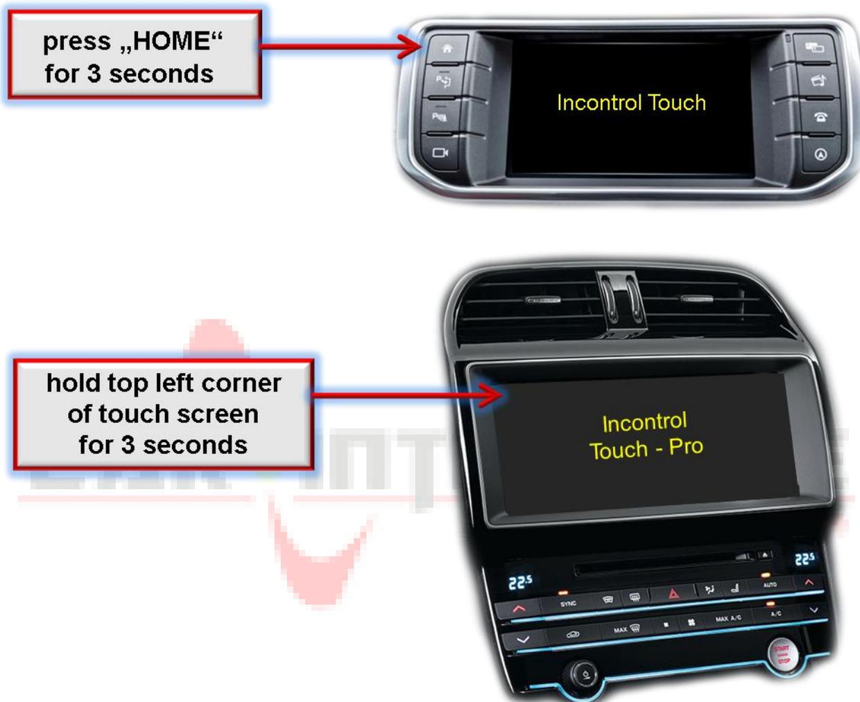
To switch the interface's activated video sources, the factory infotainment buttons can be used.
