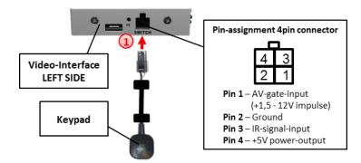
1 Connect the female 4pin connector of the keypad to the male 4pin connector of the video-interface.
