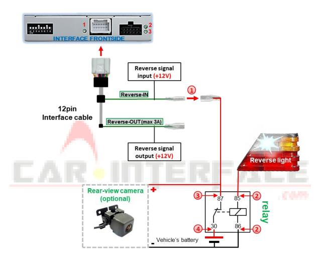
① Disconnect the green cable's pre-connected male- and female connectors of the 12pin cable and connect the green input cable "Reverse-IN" to the output connector (87) of the relay.
