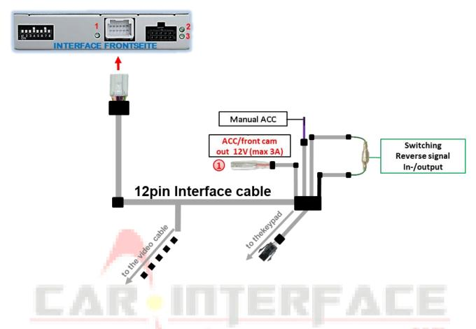
The red power supply output ACC/front cam out 12V (max 3A) can be used to power an external source and has a different assignment, depending on the position of dip switch 1 (of 8 dips):
