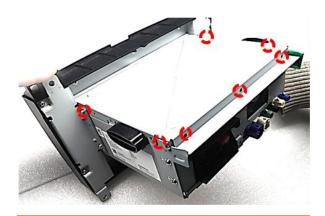
Unscrew the 7 screws at the top of the head unit and remove the housing cover.
