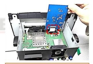
Connect the opposite side of the enclosed 40pin ribbon cable to the ribbon cable base "PCB-IN" of the daughter PCB's bottom side.
