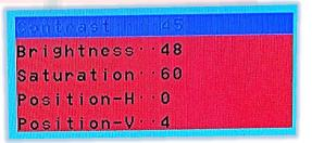
**Note:** To adjust the reverse picture settings, engage the reverse gear.
