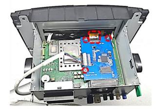
Attach the daughter PCB to the spacers. Connect the previously become free 40-pin copper-coloured ribbon cable to the ribbon cable base "LCD-OUT".
