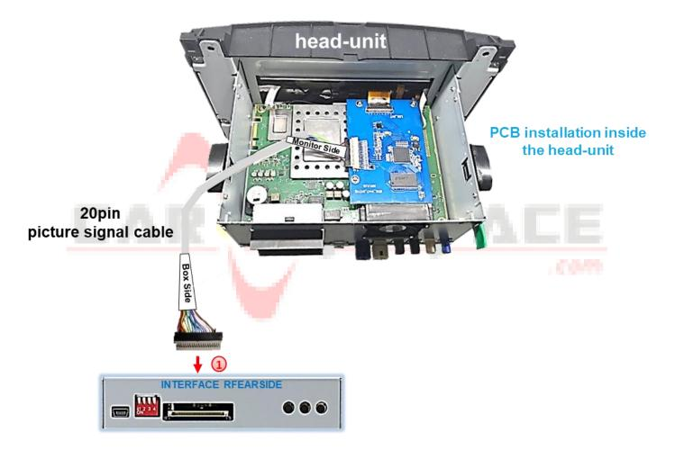
Connect the female 20pin connector of the daughter PCB's pre-connected 20pin picture signal cable to the video interface's male 20pin connector.
