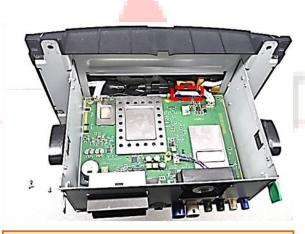
Unclick and disconnect the original copper-coloured 40pin ribbon cable from the ribbon cable base and connect the enclosed 40pin ribbon cable instead.
