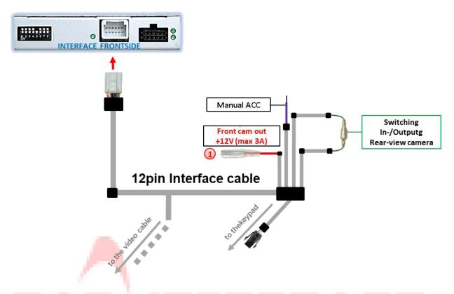
The red power supply output Front cam out +12V (max 3A) can be used to power an external source and has a different assignment, depending on the position of dip switch 1 (of 8 dips):
