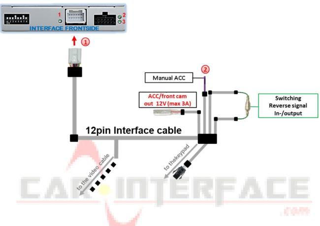
1 Connect the red wire ACC-OUT and the purple coloured wire Manual ACC of the 12pin interface cable to +12V ACC power supply.
