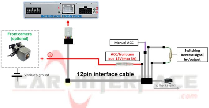
The red power supply output ACC/front cam out 12V (max 3A) can be used to power a front camera. If Dip 1 is set to ON (black 8 dips), the power supply output gives +12V (max 3A) when reverse gear is engaged plus 10 seconds delay after reverse gear is disengaged.
