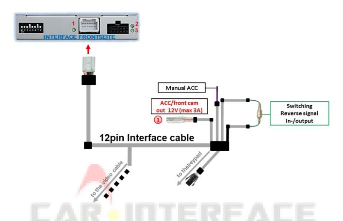
The red power supply output ACC/front cam out 12V (max 3A) can be used to power an external source and has a different assignment, depending on the position of dip switch 1 (of 8 dips):
