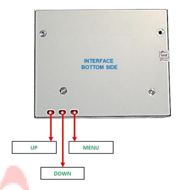
The picture settings are adjusted by the 3 buttons on the video-interface. Press the MENU button to open the OSD settings menu or to switch to the next menu item. Press UP and DOWN change the selected value. The buttons are embedded in the housing to avoid accidental changes during or after installation. Picture settings must be done separately for RGB, AV1, AV2 and CAM while the corresponding input is selected and visible on the monitor.
