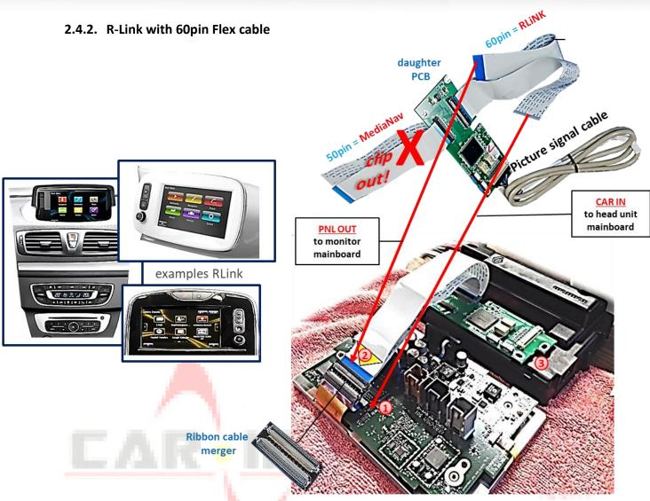
1 Remove the Ribbon cable between the monitor's monitor panel and the monitor PCB. Connect the daughter PCB's ribbon cable CAR-IN to the ribbon cable base of the main PCB. For this procedure you may either use the original ribbon cable or the ribbon cable of daughter PCB. Make sure that the connector pins of each pin connector are faced to the platinum before clipping them.
