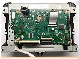
After the 40pin ribbon cable has been led out at the indicated point, mount the monitor board again and clip the 40pin ribbon cable to the ribbon cable base of the mainboard.
