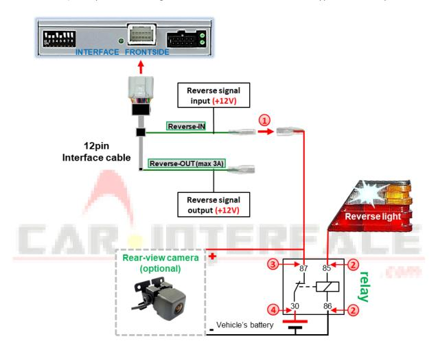
1 Disconnect the green cable's pre-connected male- and female connectors of the 20pin cable and connect the green input cable "Reverse-IN" to the output connector (87) of the relay.
