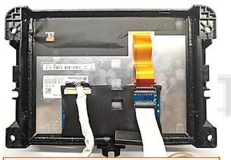
Clip out the copper-coloured 40pin ribbon cable coming from the monitor to the free ribbon cable base "CN1" of the PCB, and the enclosed 20pin picture signal cable to the 20pin ribbon cable base.
