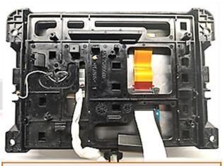
After the previously connected 20pin picture signal cable and 40pin ribbon cable have been led out at the point shown, refit the previously removed plastic housing.
