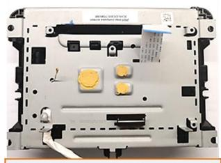
After the 40pin ribbon cable has been routed out in the position shown, refit the previously removed metal plate.
