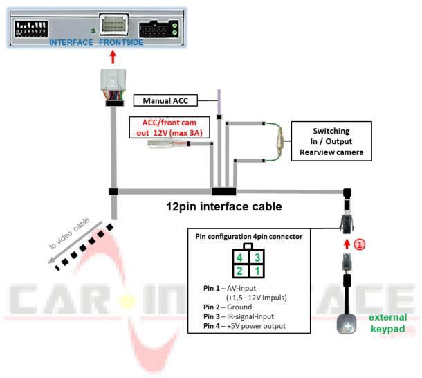
1 Connect the keypad's female 4pin connector to the 12pin interface cable's male 4pin connector.
