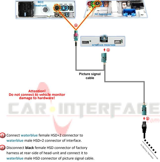
3 Connect waterblue female HSD connector to black male HSD connector at rear-side of head-unit.
