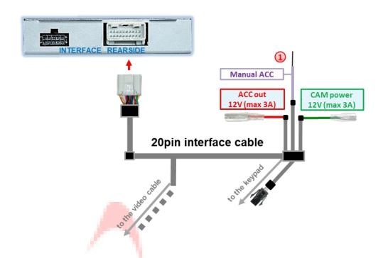
Connect purple wire Manual ACC of 20pin interface cable to +12V S-contact terminal 86s or ACC terminal 15r of vehicle (e.g., cigarette lighter, glove compartment illumination).
