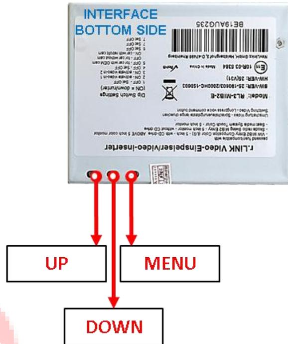
The picture settings are adjustable by the 3 push-buttons on the video-interface. Press the MENU button to open the OSD settings menu or to switch to the next menu item. Press UP and DOWN to change the selected value. The buttons are placed inside in the housing to avoid accidental changes during or after the installation. Picture settings must be done separately for AV1, AV2 and CAM while the corresponding input is selected and visible on the monitor.
