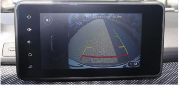
displayed on the monitor when reverse gear is engaged. Depending on the settings in the camera menu, the image is displayed in full screen mode or in split screen mode together with the factory PDC display (if present - see picture)
