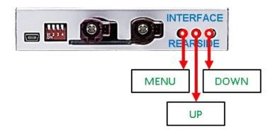
The picture settings are adjustable by the 3 push-buttons at the rear-side of the video-interface. Press the MENU button to open the OSD settings menu or to switch to the next menu item. Press UP and DOWN to change the selected value. The buttons are placed inside in the housing to avoid accidental changes during or after the installation. Picture settings must be done separately for V1, V2, V3 and V4 while the corresponding input is selected and visible on the monitor.
