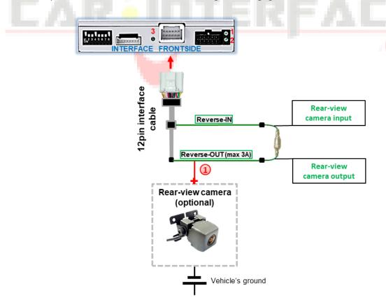
Additionally, the +12V (max. 3A) power supply for the rear-view camera can be taken from the green wire of the 12pin interface cable.
