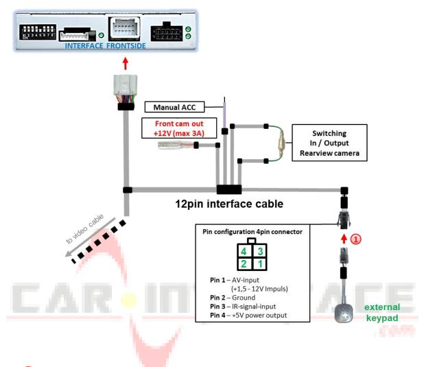
Connect the female 4pin connector of the keypad to the male 4pin connector of the 12pin interface cable.
