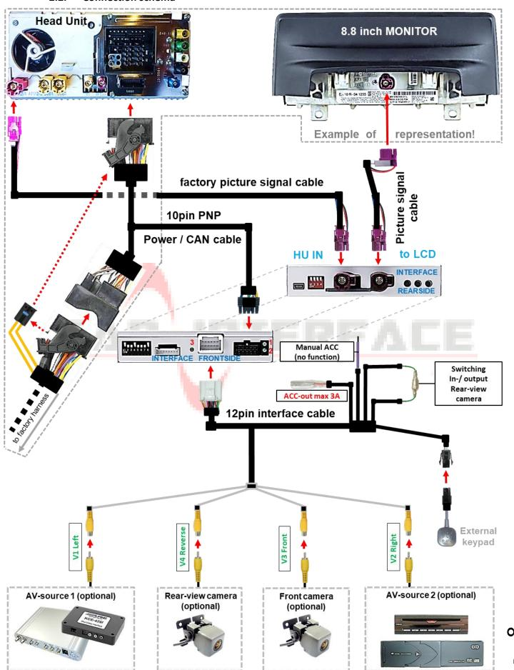
2.3. Connections to factory head-unit and monitor
