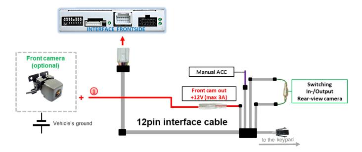
1 The red power supply output ACC/front cam out 12V (max 3A) can be used to power a front camera. If Dip 1 is set to ON (black 8 dips), the power supply output gives +12V (max 3A) when reverse gear is engaged ...
