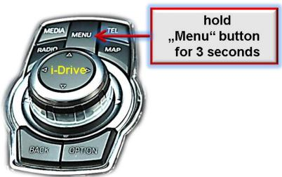
Instead of long pressing the external keypad, the MENU button of the iDrive can be long pressed to switch to V1-Left and V2-Right. Switching to V3-Front is not possible by iDrive.
