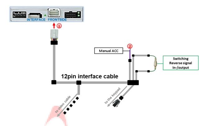
If, after connecting the PNP harness, no interface LED lightens up while the ignition is turned on, the purple-coloured wire Manual ACC of the 12pin interface cable has to be connected additionally to ACC or S-contact terminal 86s +12V (e.g. glove compartment illumination).
