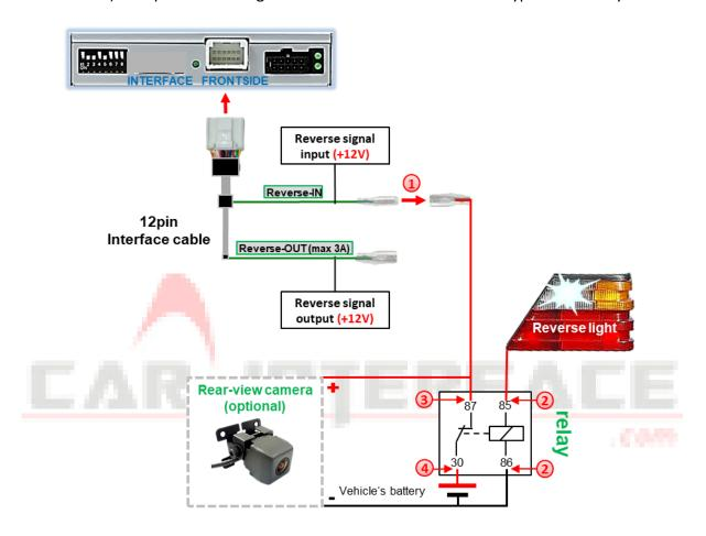
Disconnect the green cable's pre-connected male- and female connectors of the 20pin cable and connect the green input cable "Reverse-IN" to the output connector (87) of the relay.
