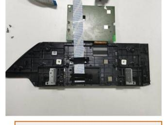
Remove the mainboard from the back of the monitor and carefully fold it upwards. Use the flex connector to connect the **longer** 50pin ribbon cable to the freed 50pin OEM ribbon cable of the monitor panel.
