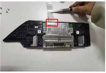
Clip the **shorter** of the two 50pin ribbon cables into the empty socket on the mainboard and thread it through the opening in the mainboard. Carefully fold back the mainboard and attach it to the back of the monitor.
