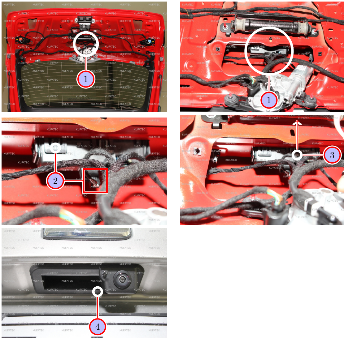
Figure 7: Disassembly button / Assembly rear view camera
