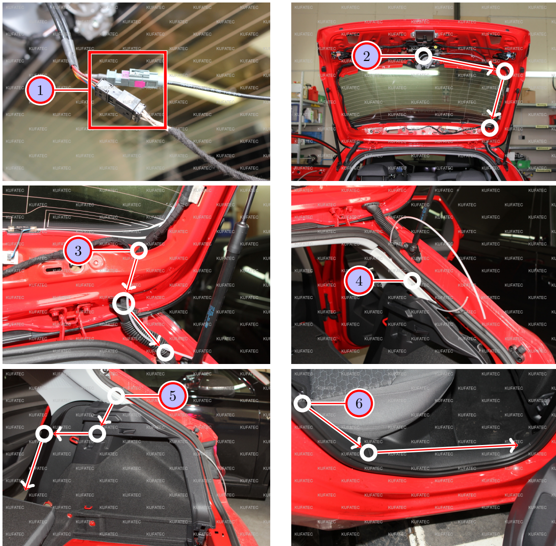
Figure 8: Cable routing tailgate to main unit
