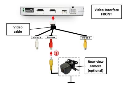
Connect the video-RCA of the after-market rear-view camera to the female RCA port of the video-interface which is labeled as CAM.
