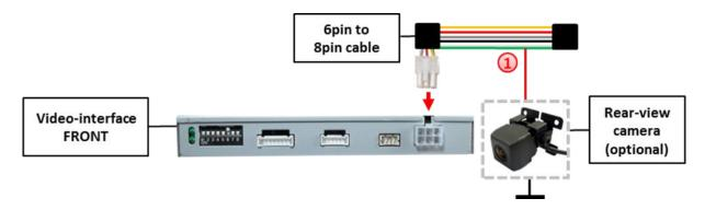
Strip a little part from the green wire of the 6pin to 8pin cable and connect it to the Power cable of the after-market rear-view camera
