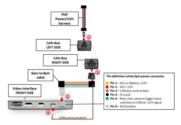
1 Connect the black female 6pin Micro-Fit connector of the PNP Power/CAN harness to the male 6pin Micro-Fit connector of the CAN-box.
