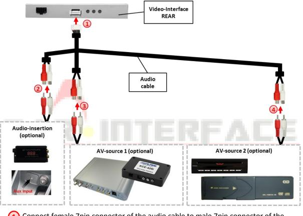
Connect female 7pin connector of the audio cable to male 7pin connector of the video-interface.
