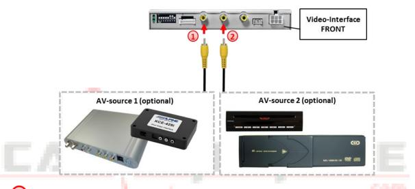
1) Connect video RCA of the AV-source 1 to the female RCA connector IN 1 of the videointerface.
