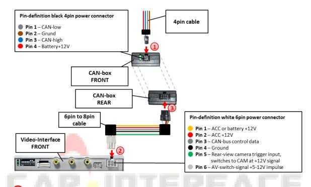
1) Connect black female 4pin Micro-Fit connector of the 4pin cable to the male 4pin Micro-Fit connector of the CAN-box.
