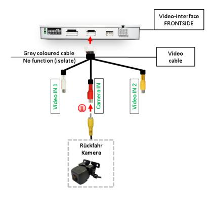
Connect the video-RCA of the after-market rear-view camera to the female RCA port of the video-interface which is labeled as CAM.
