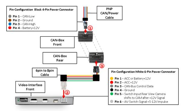
1 Connect the black female 8pin connector of the PNP Power/CAN harness to the male 8pin connector of the CAN-box.
