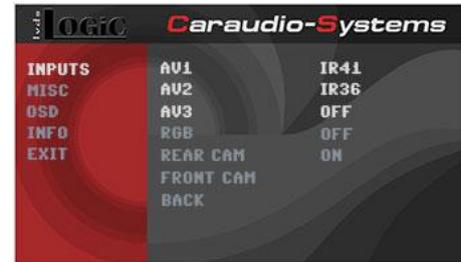
**Note:** The IR-control channel AV1 is preset to RC-Code 41 compatible DVB-T tuners and AV2 is preset to RC-Code 36 for the usbLiNK2.
