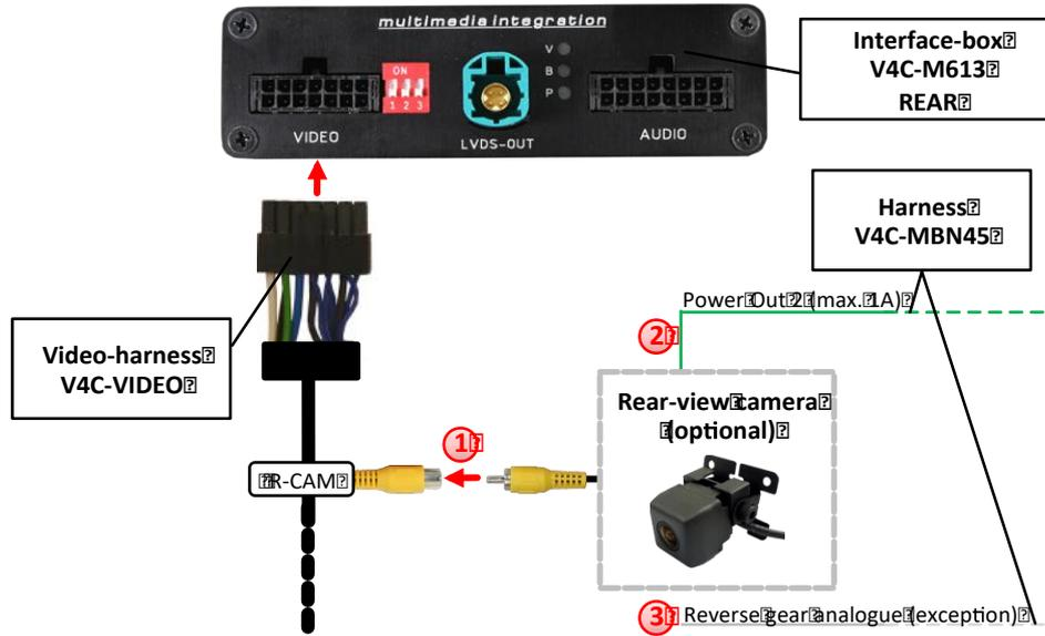
**1** Connect the video RCA of the after-market rear-view camera to the female RCA connector of the video-harness V4C-VIDEO.
