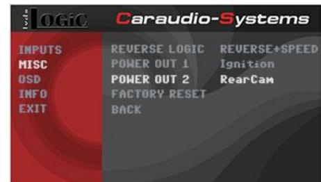
**3** On some vehicles the reverse light signal doesn’t exist on the CAN-bus. Connect the white wire of harness V4C-MBN45 to reverse light signal (+12V of reverse light) if the v.LOGiC doesn’t switch to the rear-view camera automatically after the described OSD-setup (see next chapter).
