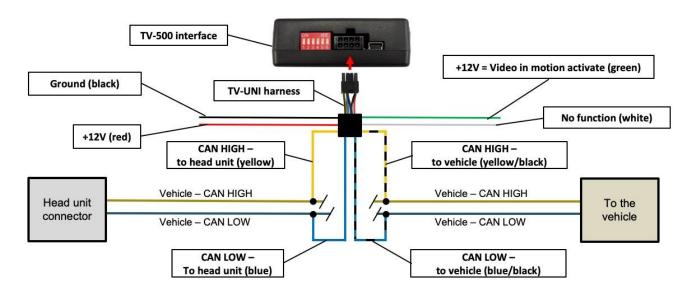
The video-in-motion can be activated and deactivated by DIP 1 or alternatively by the included loose green cable in connection with a switch (not included in delivery).\*
