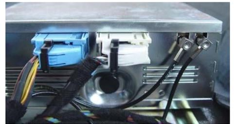
2. Remove the blue plug by repositioning the black bracket and connect it to the TV-free interface.
