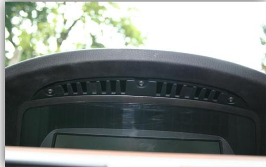
Remove cover grill (only plugged). Place soft towel beneath the board monitor to avoid scratches
