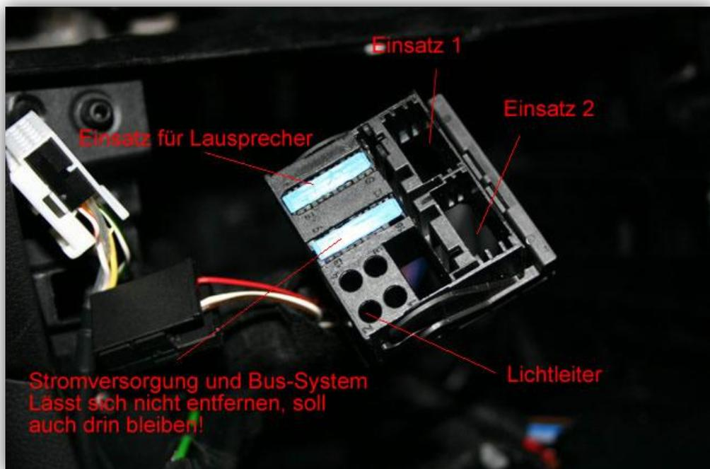
In the female Quadlock connector there is two compartments for inserts. Plug white insert of the interface harness C1C-BMW0X into compartment for "Einsatz 1".
