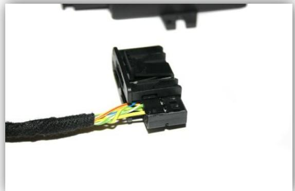
Insert completed connector into the plug on the backside of the board monitor.
