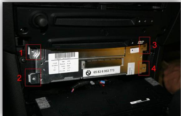
Disconnect Quadlock connector from the back of the navigation computer.
