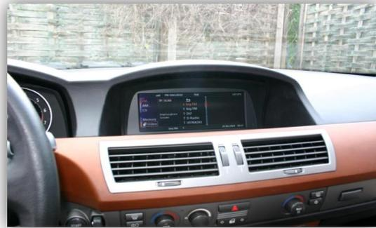
Remove 3 TORX screws at the OEM screen.
