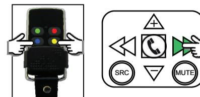
To entry into the sub-menus or to confirm a choice, please do a short pressure on the remote control on button A or, through the steering wheel commands, please do a short pressure on the SRC button. If this button is not available, please do the sequence SEEK - / SEEK +.
