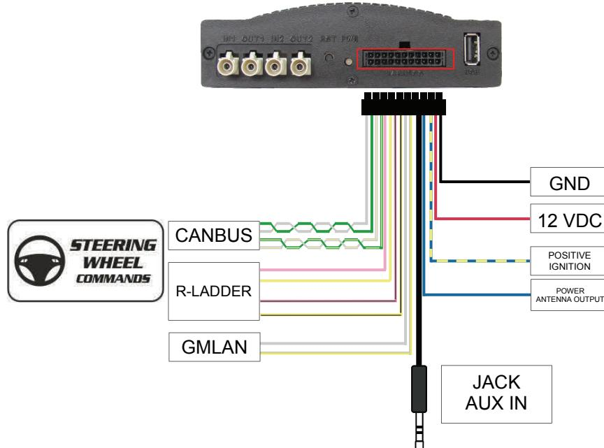
Connect steering wheel interface wires in series to the OEM wires, for example in a car that uses CANBUS protocol is necessary to cut the CAN H wire and connect GREEN wire to the car side and GREEN/YELLOW to the radio side, the same must be done with CAN L and WHITE and WHITE/YELLOW wires.
