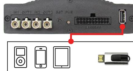
Reproduction will start automatically after the device connection, anyway it will be always possible to change the active source by the interface menu.
