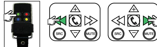
To scroll down the menu headings, the user can use the remote control indicators buttons or the steering wheel commands, by pressing the seek buttons.
