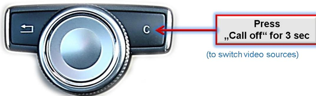
**Long press C button** (3 sec.) beside knob in centre console to switch the video source. Each repetition will switch to the next enabled input. If all inputs are enabled the order is:
