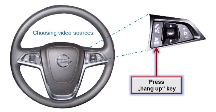
To switch the interface's activated video sources, the factory infotainment buttons can be used.
