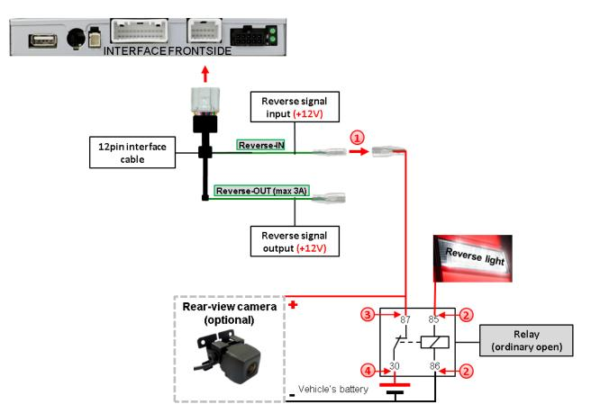
Disconnect the green cable's preconnected male- and female connectors of the 12pin interface cable and connect the green input cable "Reverse-IN" to the output connector (87) of the relay.
