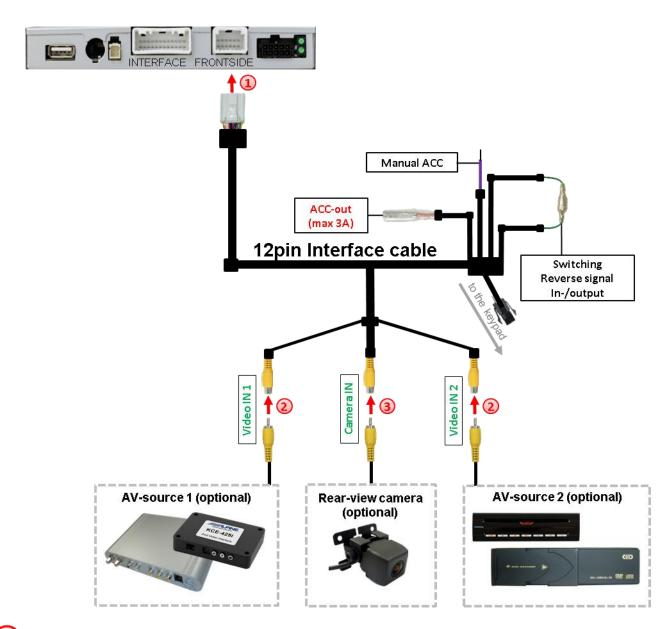
Connect the female 12pin connector of the 12pin interface cable to the male 12pin connector of the video-interface.
