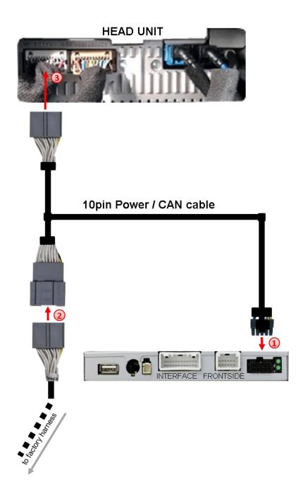
Connect the female 10pin connector of the 10pin Power / CAN cable to the 10pin connector of the video interface.
