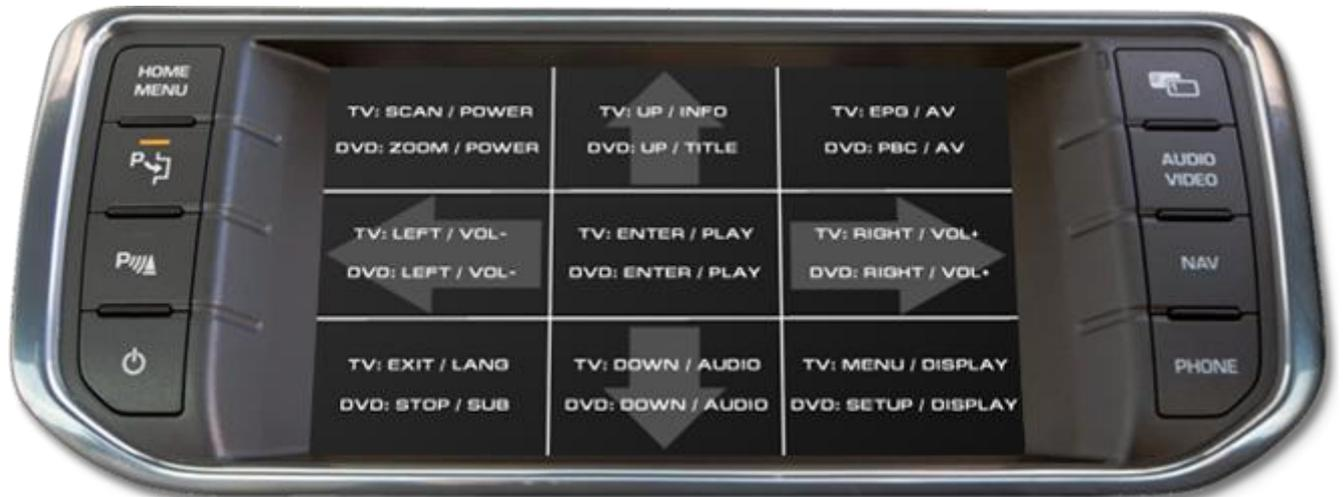
**Note:** Additionally to the control via factory touch-screen, it is possible to install the original IR-sensor of the AV-source. By using the Y-adapter STA-Y for the IR-Port of the AV-source, the controls of touch-screen AND device's IR-sensor can be connected and used simultaneously. Installation of the IR-sensor is recommended as the controls via touch-screen are limited, and not all functions may be covered.
