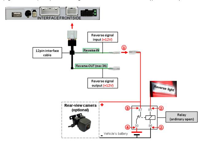
① Disconnect the green cable's preconnected male- and female connectors of the 12pin interface cable and connect the green input cable "Reverse-IN" to the output connector (87) of the relay.
