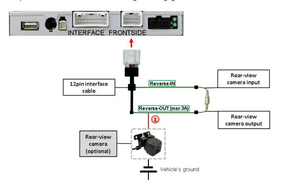
Additionally, the +12V (max. 3A) power supply for the rear-view camera can be taken from the green wire of the 12pin interface cable.
