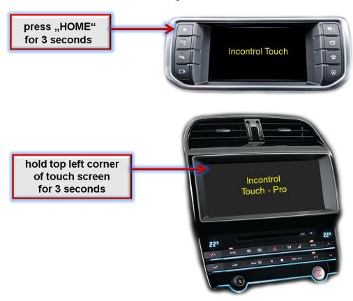
To switch the interface's activated video sources, the factory infotainment buttons can be used.
