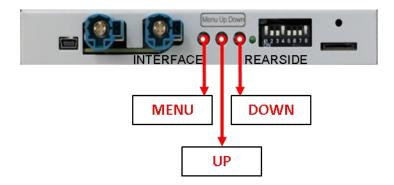
The picture settings are adjustable by the 3 push-buttons at the rear-side of the video-interface. Press the MENU button to open the OSD settings menu or to switch to the next menu item. Press UP and DOWN to change the selected value. The buttons are placed inside in the housing to avoid accidental changes during or after the installation. Picture settings must be done separately for AV1 and AV2 while the corresponding input is selected and visible on the monitor.
