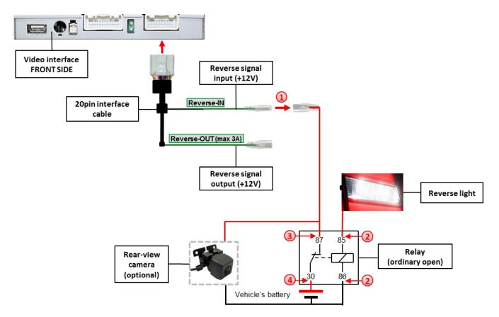
Disconnect the green cable's preconnected male- and female connectors of the 20pin cable and connect the green input cable "Reverse-IN" to the output connector (87) of the relay.
