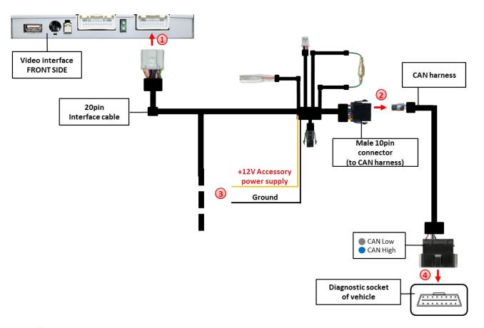
Connect the interface cable's female 20pin connector to the male 20pin connector of the video-interface.
