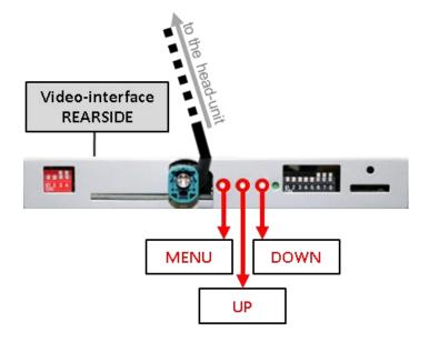
The picture settings are adjusted by the 3 buttons on the video-interface. Press the MENU button to open the OSD settings menu or to switch to the next menu item. Press UP and DOWN will change the selected value. The buttons are embedded in the housing to avoid accidental changes during or after installation. The picture settings have to be done separately for RGB, AV1 and AV2 while the corresponding input is selected and visible on the monitor.
