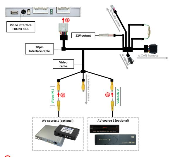
Connect the interface cable's female 20pin connector to the interface's male 20pin connector.
