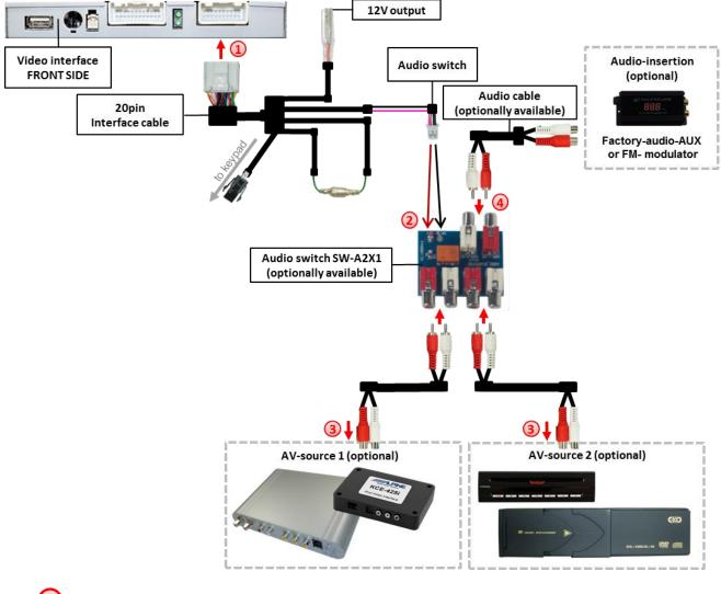
Connect the interface cable's female 20pin connector to the male 20pin connector of the video-interface.
