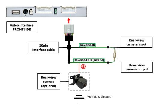
The 12 V power supply for the rear-view camera (max 3A) has to be taken from the green wire of the 20pin cable to avoid an unnecessary permanent power supply to the camera electronic.
