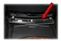
Remove the panel under the drawer (panel is slotted).
