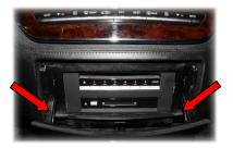
Open the drawer. Loosen the 4 Comand torx screws (2 respectively on each side).
