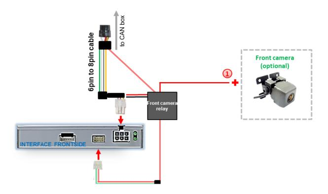
The red coloured power supply output **"Power for front"** which is coming from the front camera relay can be used to power a front camera. If Dip 6 is set to ON, the power supply output gives +12V (max 3A) when reverse gear is engaged incl. 10 seconds delay after reverse gear is disengaged.
