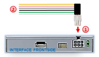
Connect the female 6pin connector of the 6pin to 8pin cable to the 6pin connector of the video interface.
