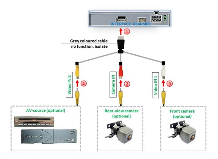
Connect the female 6pin connector of the video cable to the male 6pin connector of the video-interface.
