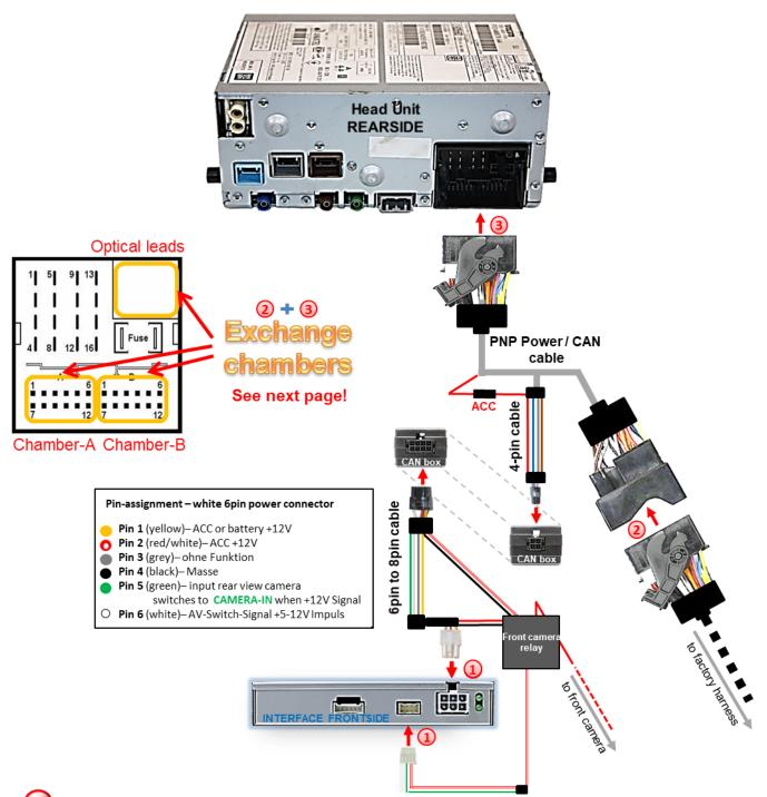
Connect the female 6pin connector of the 6pin to8pin cable to the interfaces' 6pin connector and connect the front camera relay's 8pin connector to the interfaces' 8pin connector.
