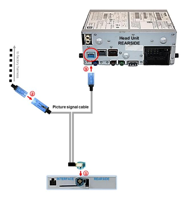
Connect the waterblue coloured female HSD+2pin connector of the picture signal cable to the male waterblue coloured HSD+2pin connector at the rear-side of the interface.
