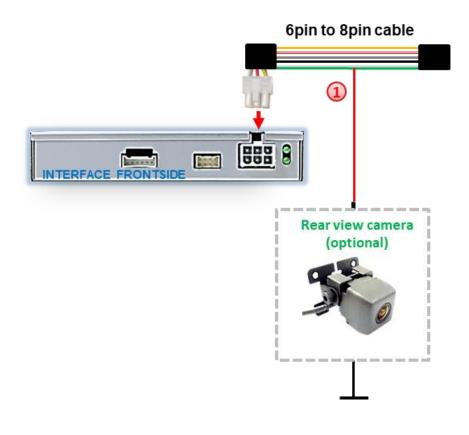
Additionally, the +12V (max. 500mA) power supply for the rear-view camera can be taken from the green wire of the 6pin to 8pin cable.
