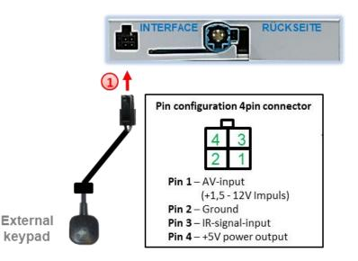
Connect the 4pin female connector of the external keypad to the male 4pin connector of the video interface.
