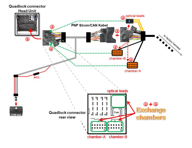
Exceptionally, the power supply to the video interfaces may not be interupted after switching to the vehicle's sleep mode. If the interface LEDs continue to shine even in the vehicle's sleep mode, separate the red wire's connection and connect the male connector to ACC or S-contact (terminal 86s)
