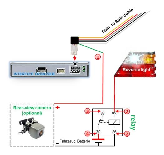
Cut the green cable of the 6pin to 8pin cable close to the black 8pin connector and isolate the shorter end of the green cable near to the 8pin connector (CAN-box side).
