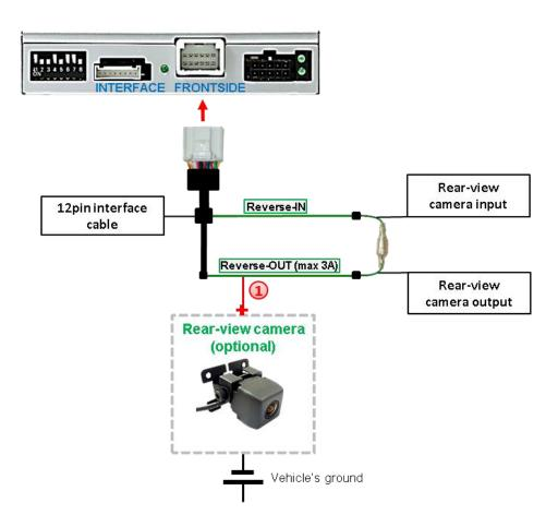
The 12 V power supply for the rear-view camera (max 3A) has to be taken from the 12pin interface cabl's green wire "Reverse-OUT" to avoid an unnecessary, permanent power supply to the camera electronic. Both green cables "Reverse IN" and "Reverse OUT" have to remain connected.
