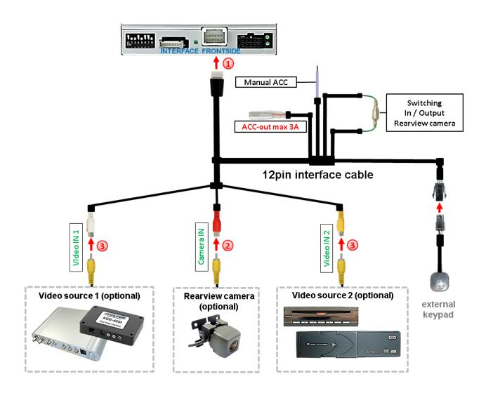
Connect the female 12pin connector of the 12pin interface cable to male 12pin connector of the video-interface.
