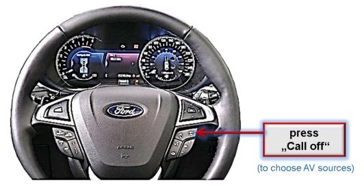
Switching the video sources can be done by a long press of the vehicle's **Call-Off button**
