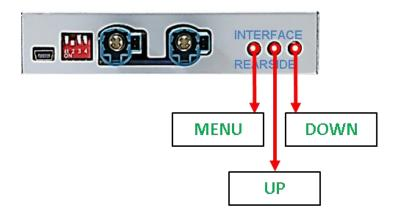
The picture settings are adjustable by the 3 push-buttons at the rear-side of the video-interface. Press the MENU button to open the OSD settings menu or to switch to the next menu item. Press UP and DOWN to change the selected value. The buttons are placed inside in the housing to avoid accidental changes during or after the installation. Picture settings must be done separately for AV1, AV2 and CAM while the corresponding input is selected and visible on the monitor.
