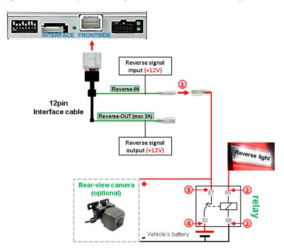
① Disconnect the green cable's preconnected male- and female connectors of the 12pin interface cable and connect the green input cable "Reverse-IN" to the output connector (87) of the relay.
