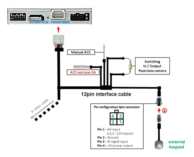
Connect the keypad's female 4pin connector to the male 4pin connector of the 12pin interface cable.
