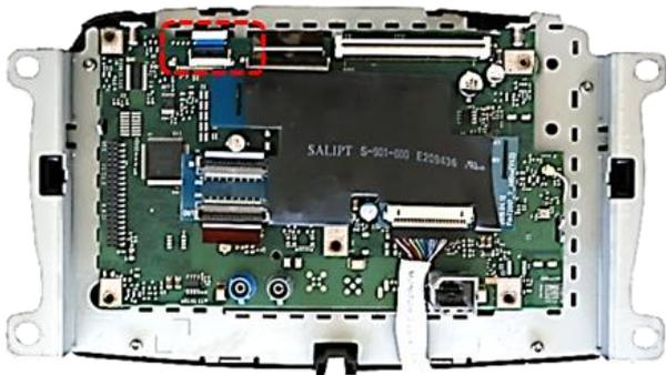
**6** Connect the enclosed 40pin ribbon cable to the mainboard's 40pin ribbon cable base and lock the connection.
