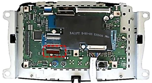
**7** Connect the previously disconnected 40pin ribbon cable to the 40pin ribbon cable base of the daughter PCB 2.
