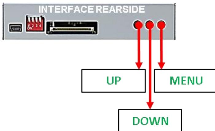
The picture settings are adjustable by the 3 push-buttons of the daughter PCB's menu keypad. Press the 1. button to open the OSD settings menu or to switch to the next menu item. By pressing the other both push buttons the selected value will be changed. To avoid accidental changes during or after the installation, we recommend to disconnect the keypad from the pushbutton cable after the adjustments are done. Adjustments have to be done, while the selected input is visible on the monitor.
