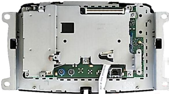
**8** Reconnect the coaxial wire between the metal brackets and fix the metal bracket. Pay attention to a perfect position of the connectors in between.
