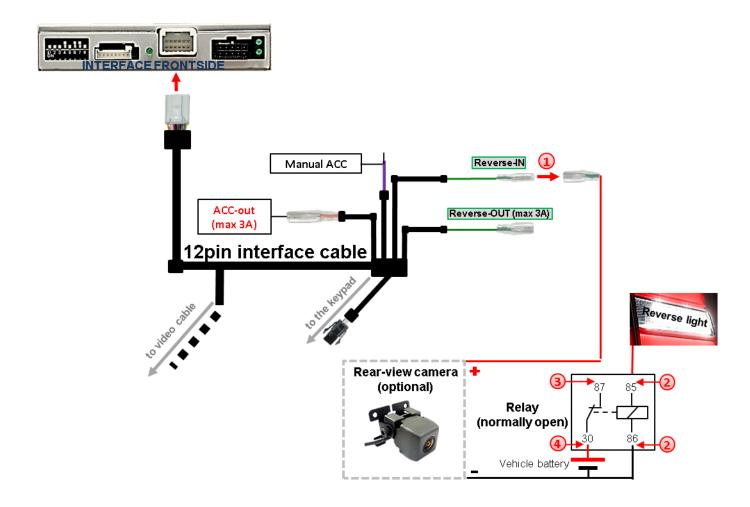
1 Disconnect the green cable's preconnected male- and female connectors of the 12pin cable and connect the green input cable "Reverse-IN" to the output connector (87) of the relay.
