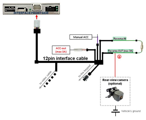
1 Additionally, the +12V (max. 3A) power supply for the rear-view camera can be taken from the green wire of the 12pin interface cable.
