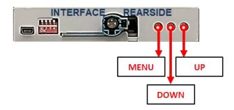
The picture settings are adjustable by the 3 push-buttons on the video-interface. Press the MENU button to open the OSD settings menu or to switch to the next menu item. Press UP and DOWN to change the selected value. The buttons are placed inside in the housing to avoid accidental changes during or after the installation. Picture settings must be done separately for Video1, Video 2 and rear-view camera while the corresponding input is selected and visible on the monitor.
