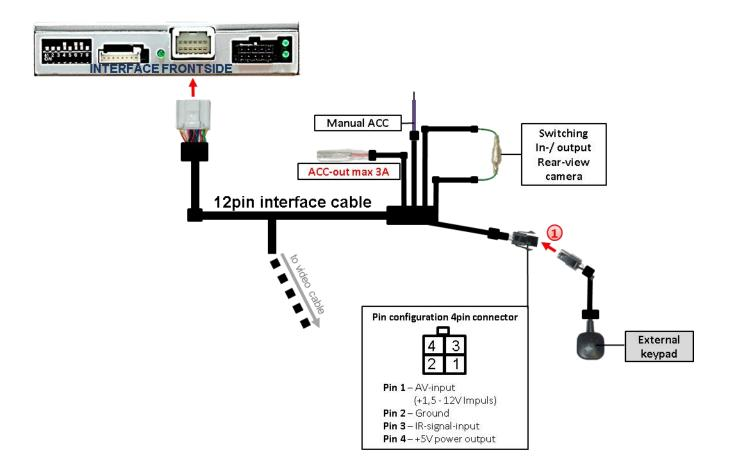
Connect the female 4pin connector of the keypad to the male 4pin connector of the 12pin interface cable.
