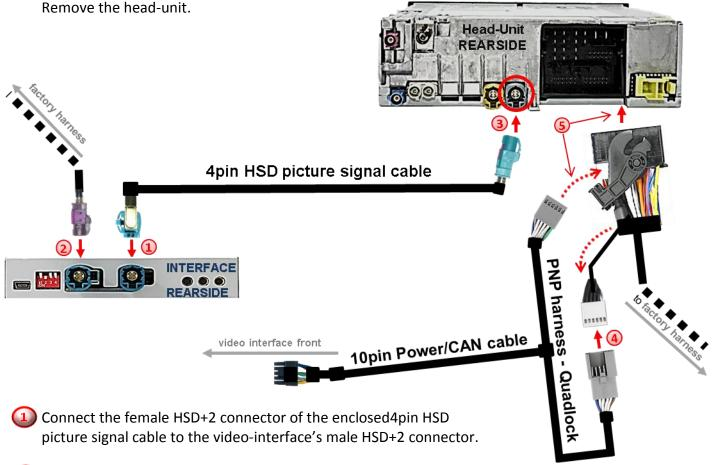
Disconnect the female 4pin HSD connector of the vehicle harness at the Rear-side of the head-unit and connect it to the interface's male 4pin HSD connector.
