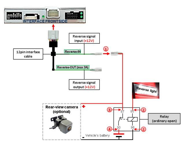
Disconnect the green cable's preconnected male- and female connectors of the 12pin cable and connect the green input cable "Reverse-IN" to the output connector (87) of the relay.
