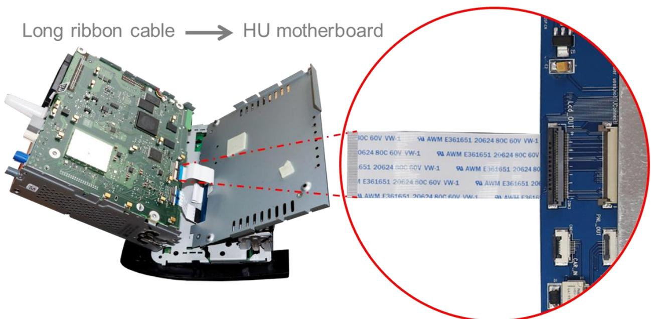
After a check of the perfect ribbon cable connection, in reverse order fold back and clip in the head-unit housing to the head-unit control panel and fix the exchange housing base plate to the head-unit's housing.
