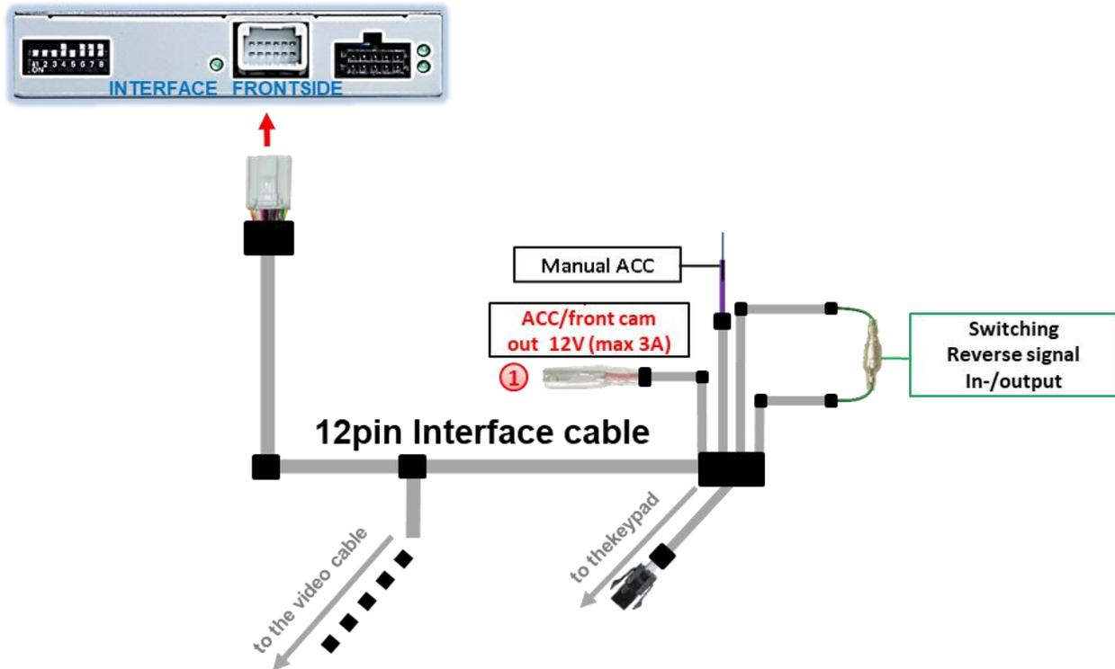
① The red power supply output **ACC/front cam out 12V (max 3A)** can be used to power an external source and has a different assignment depending on the position of dip switch 1 (of the black 8 dips):
