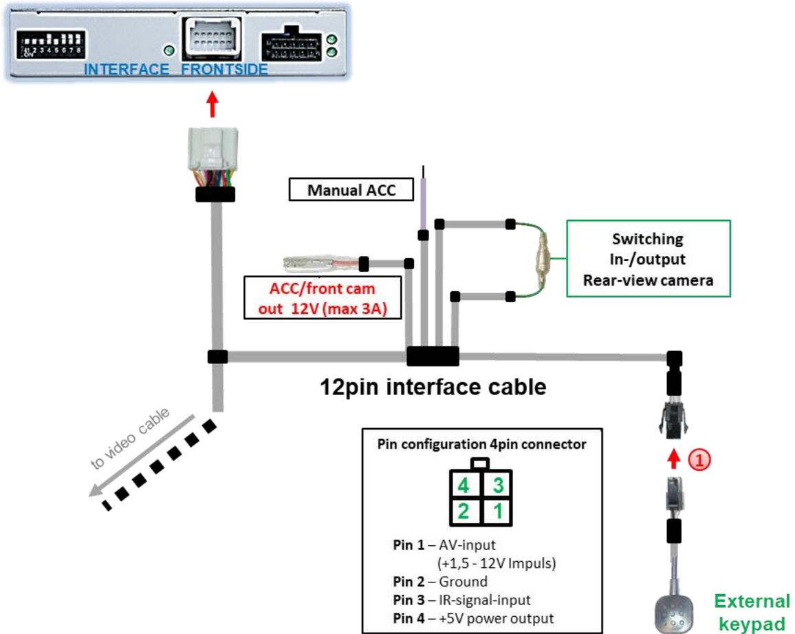
① Connect the keypad’s female 4pin connector to the 12pin interface cable’s male 4pin connector.
