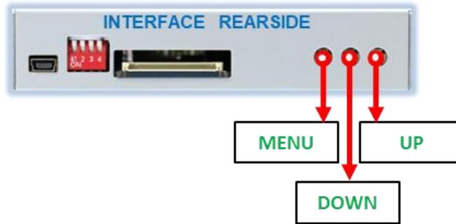
The picture settings can be adjusted by the 3 buttons on the video-interface. Press the **MENU** button to open the OSD settings menu. To switch to the next menu item, pressing **UP** and **DOWN** will change the selected value. The buttons are embedded in the housing to avoid accidental changes during or after installation. The picture settings have to be done separately, AV1 and AV2 while the corresponding input is selected and visible on the monitor.
