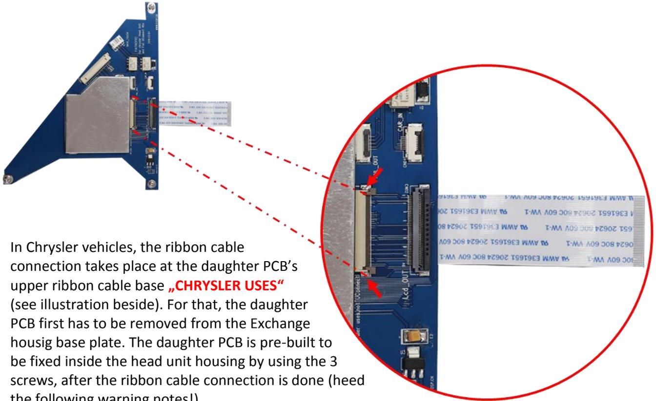
In Chrysler vehicles, the ribbon cable connection takes place at the daughter PCB's upper ribbon cable base „**CHRYSLER USES**“ (see illustration beside). For that, the daughter PCB first has to be removed from the Exchange housing base plate. The daughter PCB is pre-built to be fixed inside the head unit housing by using the 3 screws, after the ribbon cable connection is done (heed the following warning notes!).
