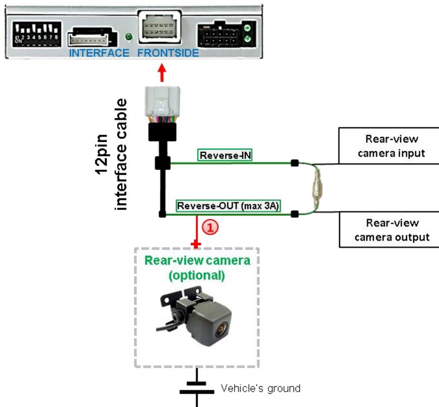
**1** Additionally, the +12V (max. 3A) power supply for the rear-view camera can be taken from the green wire of the 12pin interface cable.
