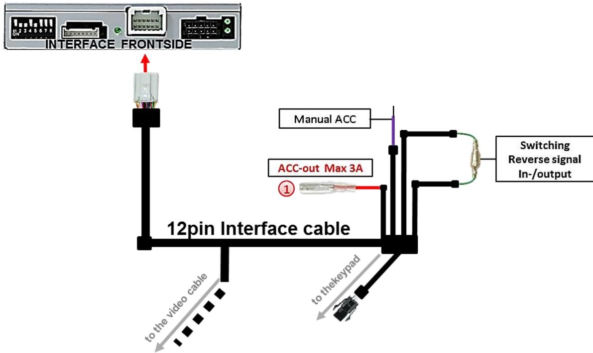
① The red power supply output **ACC-out Max 3A** can be used to power an external source (max 3A).
