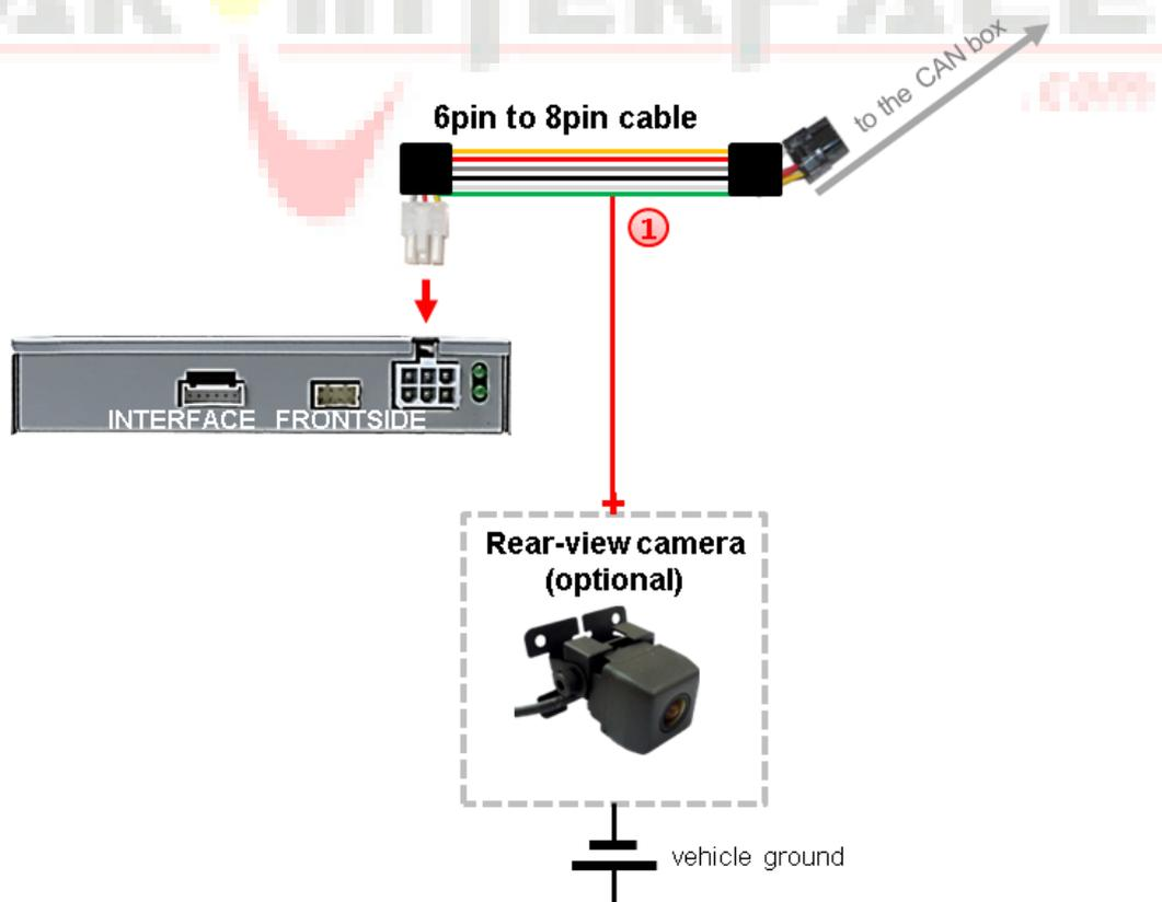
① Additionally, the +12V (max. 500mA) power supply for the rear-view camera can be taken from the green wire of the 6pin to 8pin cable.
