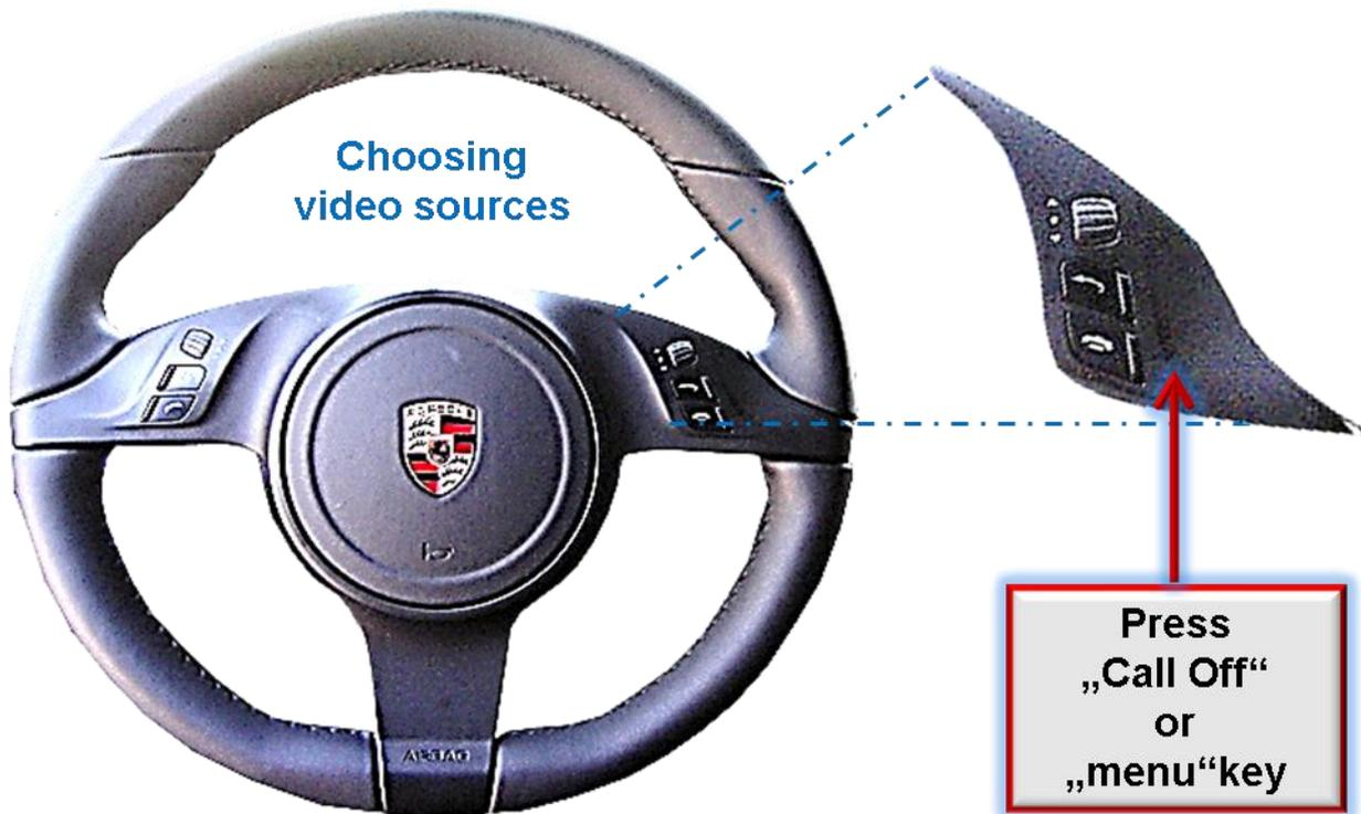
To switch the video sources the vehicle's **Call off button** or **menu button** can be used.
