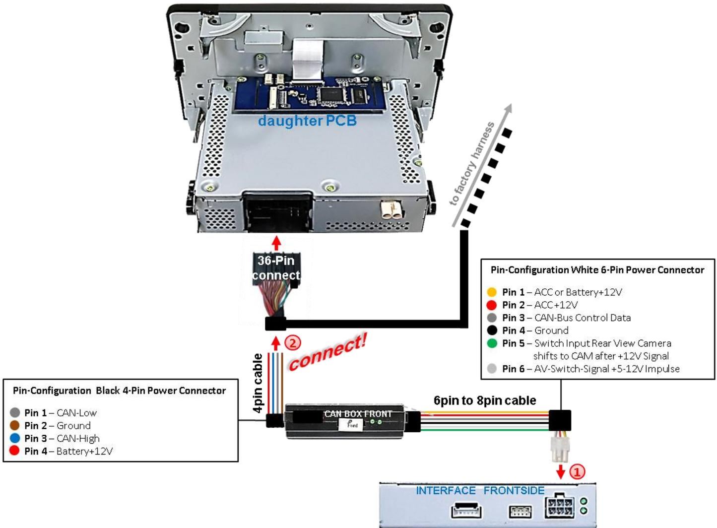
① Connect the white female 6pin connector of the 6pin to 8pin cable to the male 6pin connector of the video interface.
