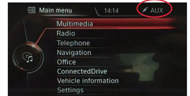
**NOTE!** Make sure source switch to "AUX" mode on original car stereo for audio transmission before using the integration.
