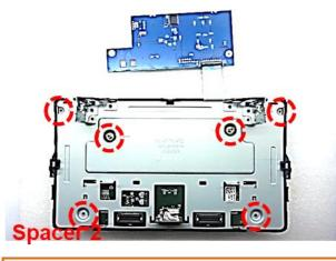
Close the monitor housing with the metal bracket and fix it with 4 of the original screws at the edges. The 2 enclosed spacers have to be screwed in the 2 free middle holes for the daughter PCB's fixing.
