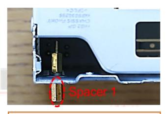
For later attachment of the daughter PCB to the Head Unit, mount one of the spacers supplied on the outside and fix it on the inside at the position shown. **See also Fig. 5**
