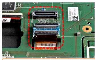
Unclip the copper-coloured factory ribbon cable from the ribbon cable base of the monitor board and clip it to the ribbon cable base of the enclosed ribbon cable merger (pre-assembled).
