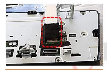
Before leading out the ribbon cables, the ribbon cable merger and the ribbon cables have also to be protected with tape to prevent cable damage and short circuits.
