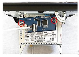
Screw the monitor to the top and bottom of the head unit, using the original screws and attach the daughter PCB to the pre-mounted spacers.
