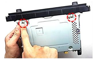
Screw out the two fixing screws at the head unit's bottom side.
