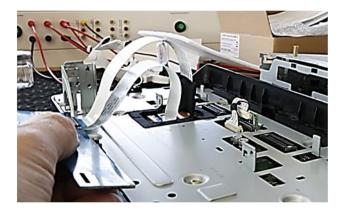
Connect the daughter PCB's ribbon cable "OUT" to the factory monitor board's cable base and connect the factory ribbon cable to the daughter PCB's cable merger "IN".
