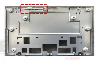
Bend the marked point on the back plate inwards to ensure that the ribbon cables are led out without injury. Additionally protect the cables with tape against injury by housing parts.
