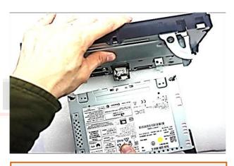
Carefully separate the monitor part from the head unit.
