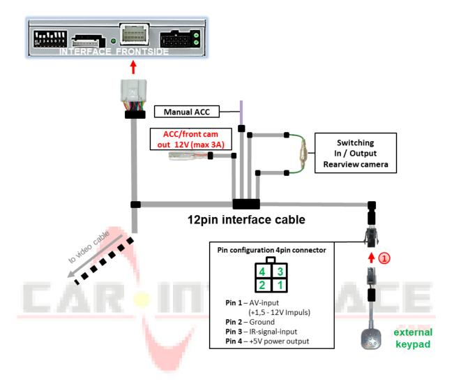
Onnect the keypad's female 4pin connector to the 12pin interface cable's male 4pin connector.
