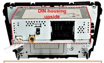
If the DIN housing is mounted on top (e.g. Skoda Rapid), the routing of the ribbon cables and the PCB installation differs. First disconnect the topmounted DIN housing from the monitor.
