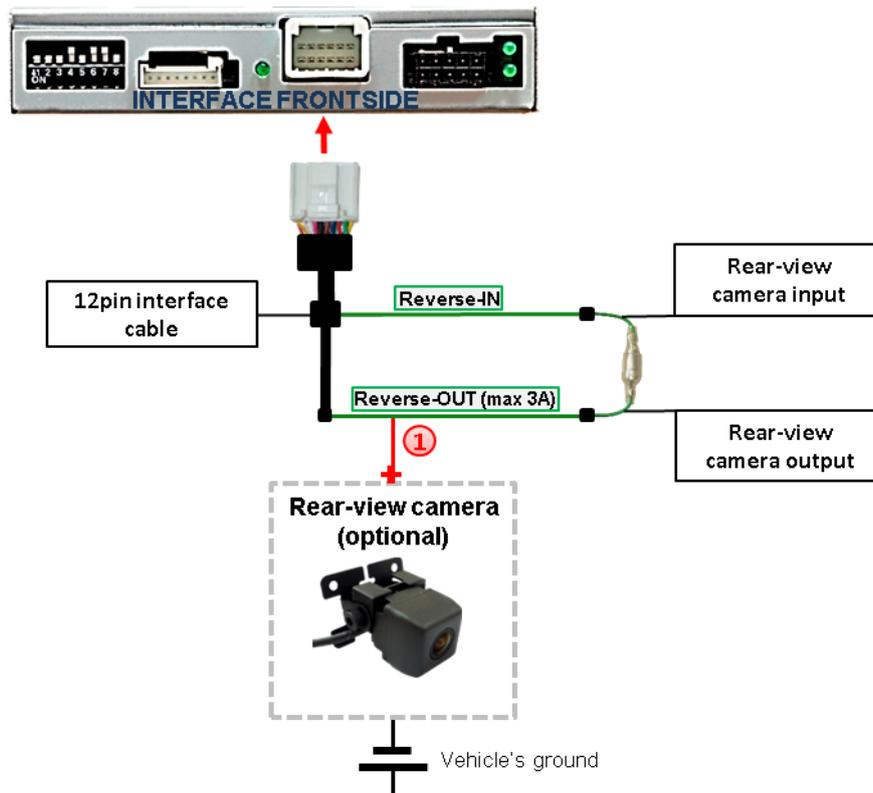
① Additionally, the +12V (max. 3A) power supply for the rear-view camera can be taken from the green wire of the 12pin interface cable.
