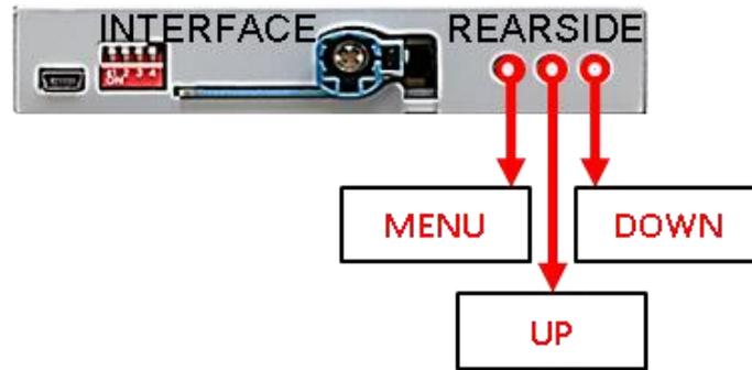
The picture settings are adjustable by the 3 push-buttons on the video-interface. Press the MENU button to open the OSD settings menu or to switch to the next menu item. Press UP and DOWN to change the selected value. The buttons are placed inside in the housing to avoid accidental changes during or after the installation. Picture settings must be done separately for AV1 and AV2 while the corresponding input is selected and visible on the monitor.
