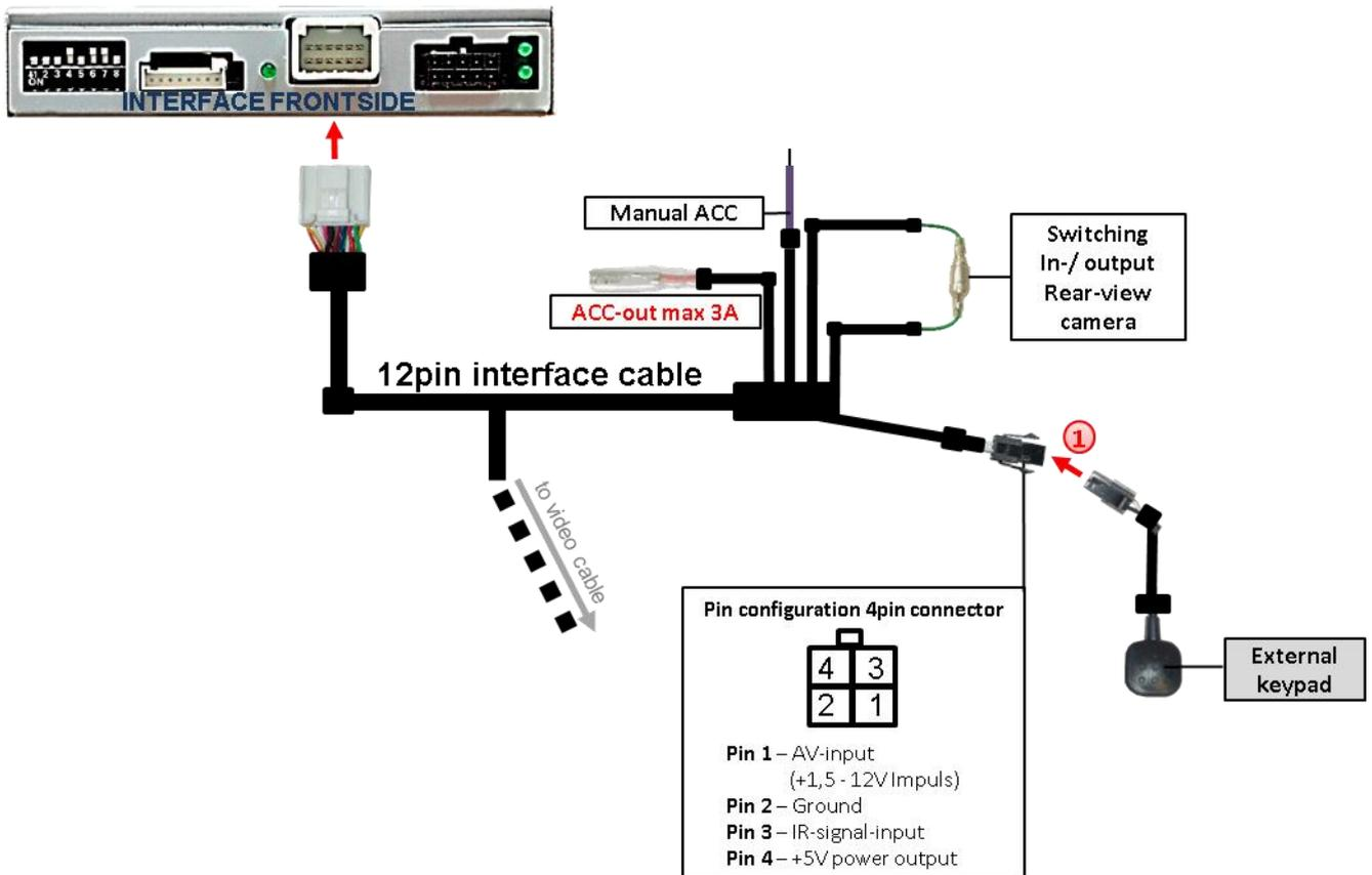
1 Connect the female 4pin connector of the keypad to the male 4pin connector of the 12pin interface cable.
