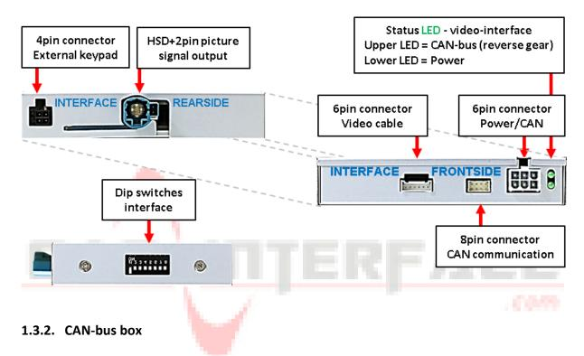
The CAN box reads the vehicle's digital signals out of the vehicle's CAN-bus and converts them for the video interface.
