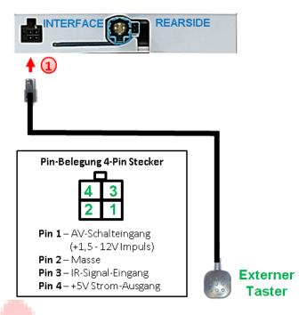
1 Connect the keypad's female 4pin connector to the video-interface's male 4pin connector.
