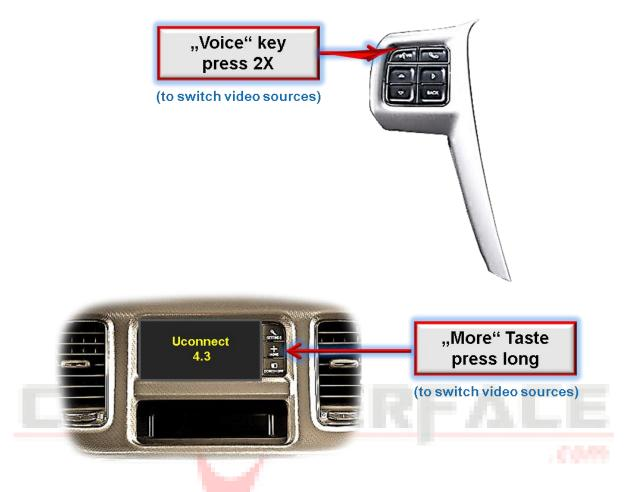
To switch the video sources the vehicle's **VOICE** button at the steering wheel or, in case of the 4.3inch monitor, the **MORE** button can be used.
