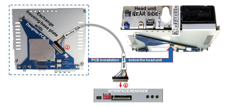
Connect the 20pin RGB digital cable's female 20pin connector to the male 20pin connector of the video-interface.
