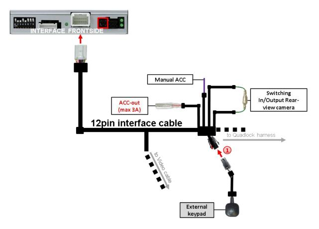
Connect the keypad's female 4pin connector to the video-interface's male 4pin connector.
