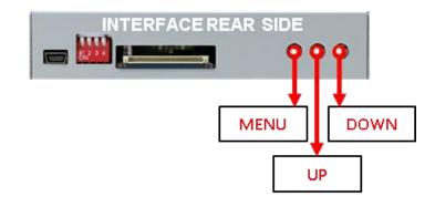
The picture settings can be adjusted by the 3 buttons on the video-interface. Press the **MENU** button to open the OSD settings menu. To switch to the next menu item, pressing UP and **DOWN** will change the selected value. The buttons are embedded in the housing to avoid accidental changes during or after installation. The picture settings have to be done separately, AV1 and AV2 while the corresponding input is selected and visible on the monitor.
