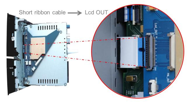
Connect the daughter PCB's pre-assembeled 40pin ribbon cable to the previously become free ribbon cable base of the head-unit mainboard. (heed the following warning notes!).
