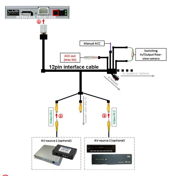
Connect the interface cable's female 12pin connector to the interface's male 12pin connector.
