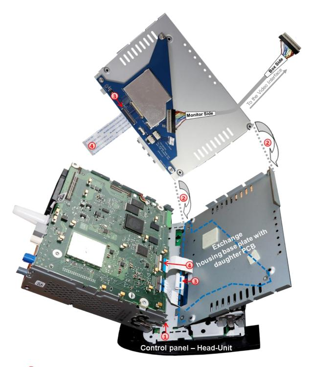
Clip out the head-unit housing at the head-unit control panel and fold it to the side, like shown in the picture above.
