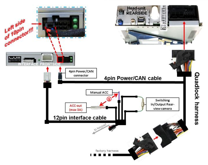
If, after connecting the 20-Pin PNP harness, no interface LED lightens up while the ignition is turned on, the single red wire ACC-out (max 3A) and the purple coloured wire Manual ACC of the 12pin interface cable both have to be connected additionately to +12V S-contact terminal 86s (e.g. glove compartment illumination).
