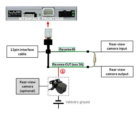
The 12 V power supply for the rear-view camera (max 3A) has to be taken from the green wire of the 20pin cable to avoid an unnecessary permanent power supply to the camera electronic.
