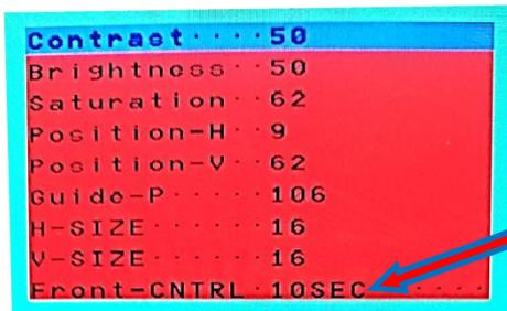
Incl. 10, 15, or 20 seconds delay after reverse gear is disengaged (refer also to chapter „picture settings“).
