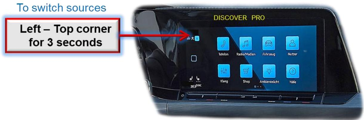
A long press in the touch display's left upper edge switches the interface's activated video sources.
