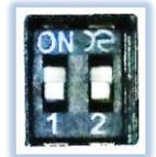
The 2 dip-switches on the upper side of the interface box are used to select the head unit. If no image is displayed, switch **both** dip-switches **PARALLEL** to the opposite position.
