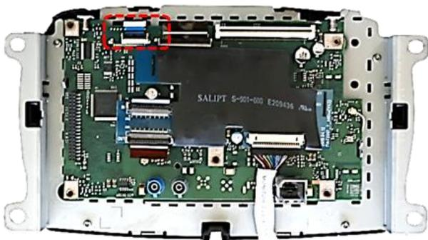
**6** Connect the enclosed 40pin ribbon cable to the mainboard's 40pin ribbon cable base and lock the connection.
