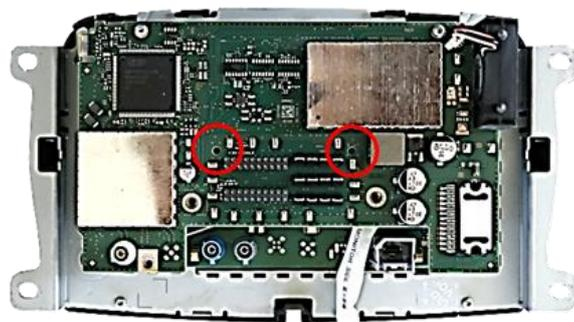
**9** Reinstall the original mainboard and fix it with the original screws
