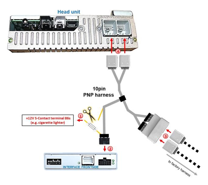
Out the yellow wire of the PNP harness near the 10pin connector and connect it to the vehicle's +12V S-contact terminal 86s (e.g. cigarette lighter)
