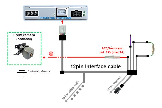
The red power supply output ACC/front cam out 12V (max 3A) can be used to power a front camera. If Dip 1 is set to ON (of the black 8 dips), the power supply output gives +12V (max 3A) when reverse gear is engaged incl. 10 seconds delay after reverse gear is disengaged.
