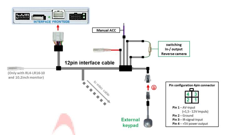
Onnect the keypad's female 4pin connector to the male 4pin connector of the 12pin interface cable.
