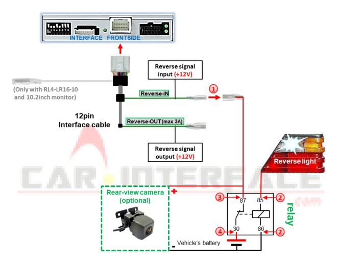
① Disconnect the green cable's preconnected male- and female connectors of the 12pin interface cable and connect the green input cable "Reverse-IN" to the output connector (87) of the relay.
