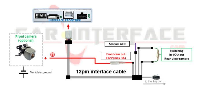
1 The red power supply output ACC/front cam out 12V (max 3A) can be used to power a front camera. If Dip 1 is set to ON (of the black 8 dips), the power supply output supplies +12V (max 3A) when the reverse gear is engaged and additionally 10 seconds delay after the reverse gear is disengaged.
