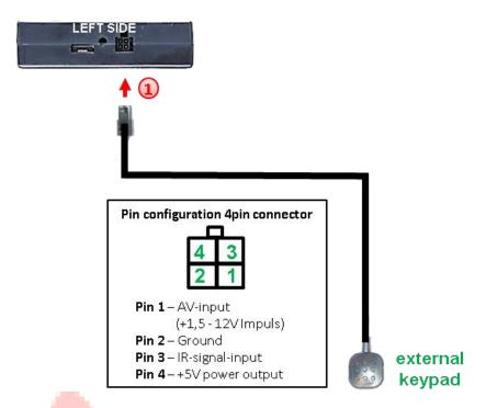
1 Connect the keypad's female 4pin connector to the video-interface's male 4pin connector.
