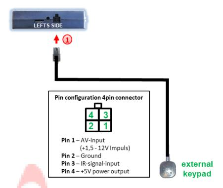
Connect the keypad's female 4pin connector to the video-interface's male 4pin connector.
